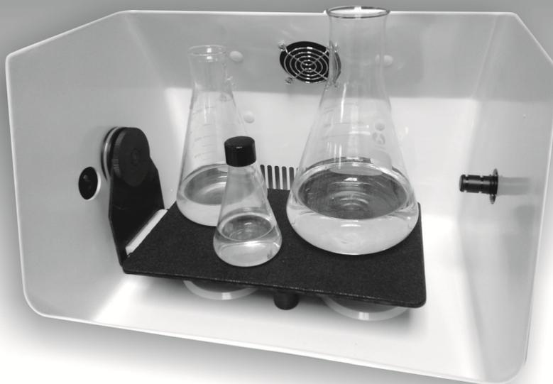
1. Place the Orbital Shaker Attachment inside the Enviro-Genie® or Incubator-Genie® chamber, aligning the hex shaft with the hex on the pulley of the Orbital Shaker Attachment. Make sure the two feet are in contact with the chamber base.
